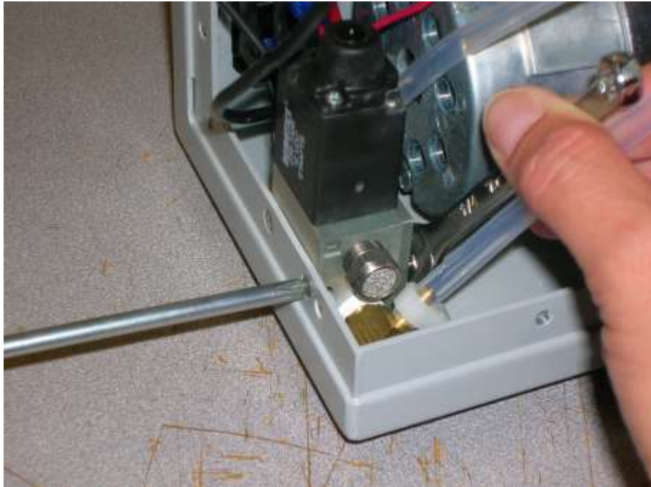
Figure 4-2: Removing solenoid from casing
